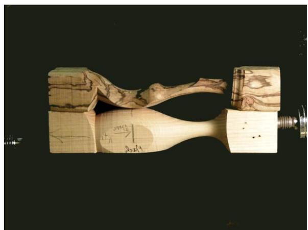
Figure 10 Profiles Compared to Master
